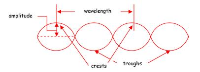
Frequency is # of wavelengths/second Frequency for this standing wave is  $4f_o$
