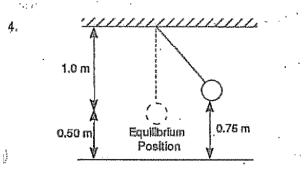
The bob of a pendulum has a mass of 2.0 kg. This bob is pulled sideways so that it is 0.75 m above the table top. What is the potential energy of the bob with respect to the equilibrium position?
