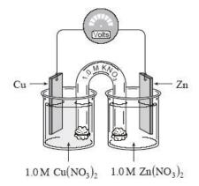
Which of the following represents the relationship between  $[NO_3^-]$  and the mass of the Cu electrode in the copper half cell as it operates?
